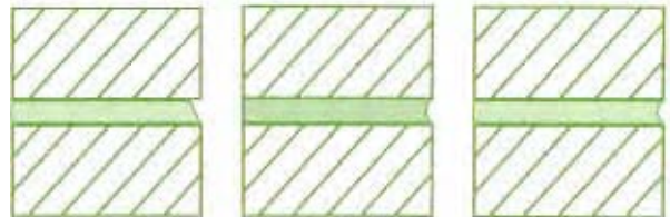
Weathered Angle Joint
